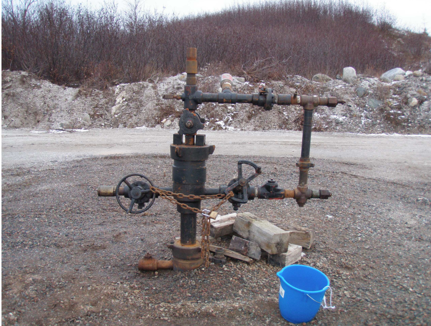
Wellhead configuration after re-entry
