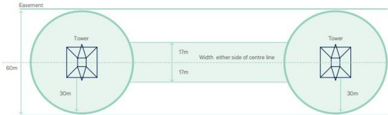
Figure 2.11: Transmission Line Easement
